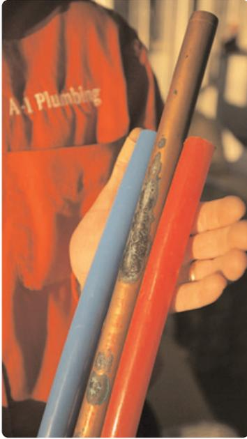
Uponor PEX tubing is highly durable and resists corrosion from aggressive water and soil conditions that cause pinhole leaks in copper pipe.
