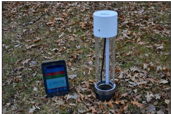
The new Modified Philip Dunne (MPD) Infiltrometer from New Brighton, Minn.-based Upstream Technologies provides an innovative solution for measuring soil absorption, eliminating water waste and benefitting the environment.
