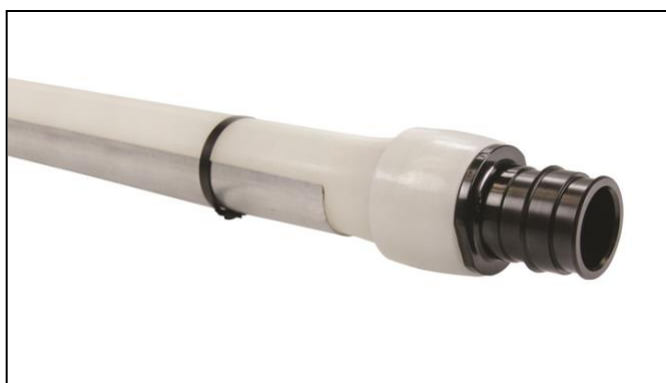
Uponor PEX-a Pipe Support is a galvanized steel channel that provides continuous support of PEX in suspended piping applications, enabling hanger spacing similar to that of copper or steel pipe.
