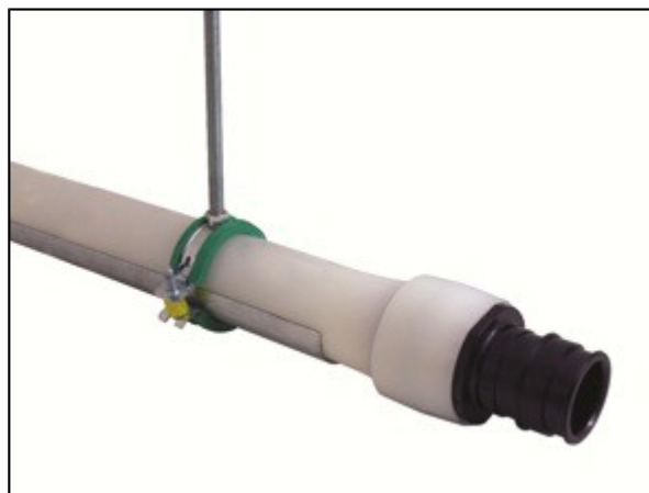
Uponor PEX-a Pipe Support is a steel channel that provides continuous support of PEX tubing in suspended piping applications, enabling hanger spacing equal to that of copper.
